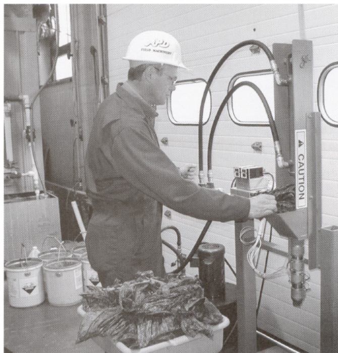
James Garthe feeds mulch film made from very dirty, plastic drip irrigation tubing into the prototype Plastofuel machine. A hydraulic cylinder forces the plastic items through a heated die, shown on the lower right. The extruded material is then cut with a hot knife to form Plastofuel, shown below.
