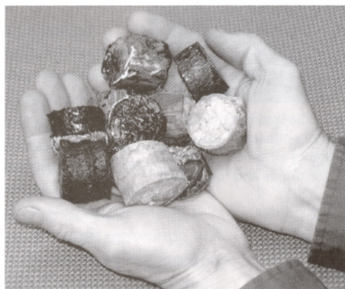
Plastofuel nuggets are made from various types of dirty plastics mixed together. The process works well using either discarded films (e.g., mulch, greenhouse, or forage), rigid plastic items (e.g., pots, trays, or flats), or both.
